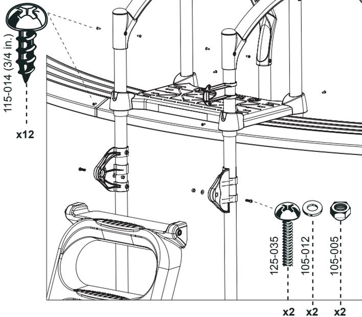
1) Secure the handrails and platform to the posts with the screws provided.
