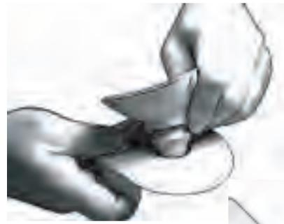
1) Insert half of the Step Cup™ mushroom in the hole, at a 45 degree angle.
